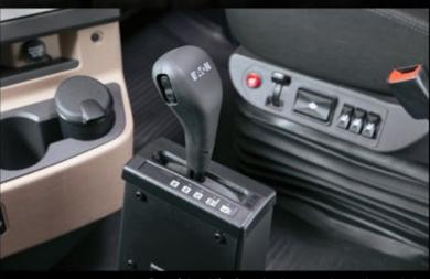
Eaton Cobra shifter for optional automated manual transmission.
