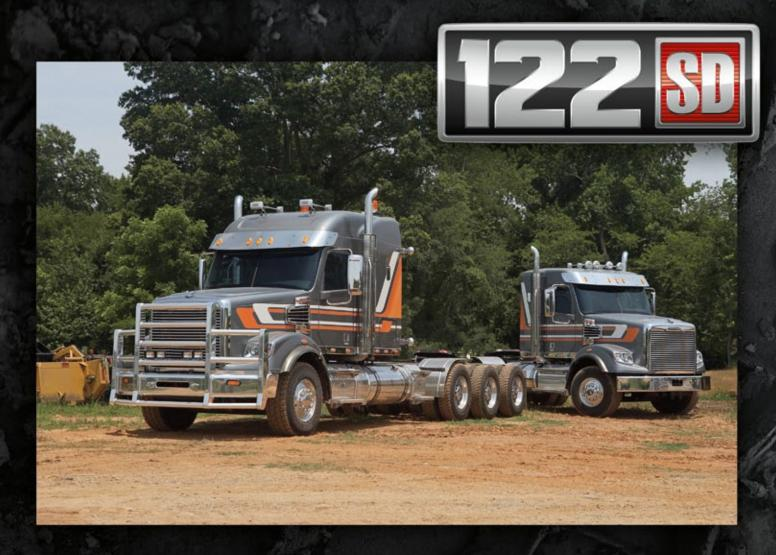
Some jobs are bigger than others. You may be hauling logs down a forest road. Or transporting an oversize load across the Alaskan wilderness. Whatever the job, it's critical to have a truck that can handle it without fail. The Freightliner Trucks 122SD is our largest severe duty truck, providing up to 600 horsepower and 2,050 lb-ft of torque at 1100 RPM. And its GCWR is rated up to 160,000 lbs. So this truck doesn't shy away from a challenge any more than you do.
