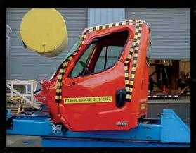
Components, systems and entire vehicles are subjected to an array of virtual and physical tests to ensure our trucks deliver the expected function, performance and reliability.
