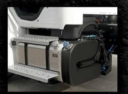
Up to two batteries located under cab for easy body upfit.
